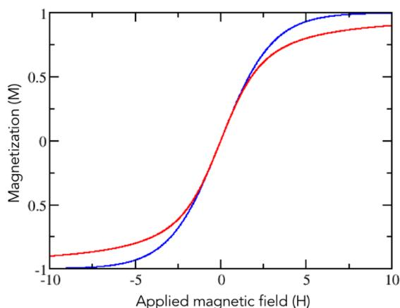
**Figure 2 – Langevin curve for the RELAX experiment.** When  $H$  is highly negative, the magnetization  $M$  starts in a saturated state. As  $H$  is increased (from left to right),  $M$  desaturates to reach a linear transition with  $H$  around 0. As  $H$  continues to increase,  $M$  re-saturates to the same intensity with opposite polarization. The same process occurs when  $H$  decreases (from right to left). Image from [2].
