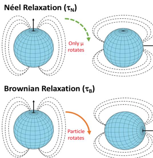
*Figure 1 - Difference between Néel and Brownian relaxation. Néel relaxation is a change in the magnetization of the particle (without movement), while Brownian relaxation is a physical rotation of the particle without a change in the internal magnetization of the particle. (adapted from [1]).*
