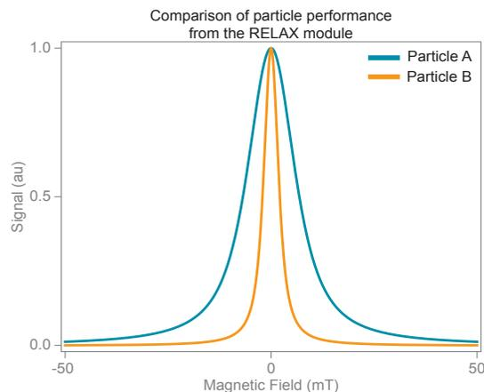
**Figure 3 – Peak-height normalized RELAX curve for 2 different particles.** In this case, particle B has a much greater intrinsic resolution because of its smaller FWHM.
