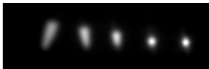
Figure 2 - Slice image of volume acquisition (Synomag®-D) showing the same amount of iron in different dilution volumes. The characteristic shape of Eppendorf's tube is clearly visible.
